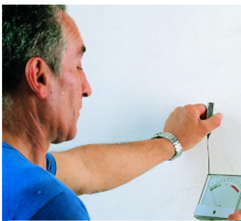
Checking gypsum plaster humidity
